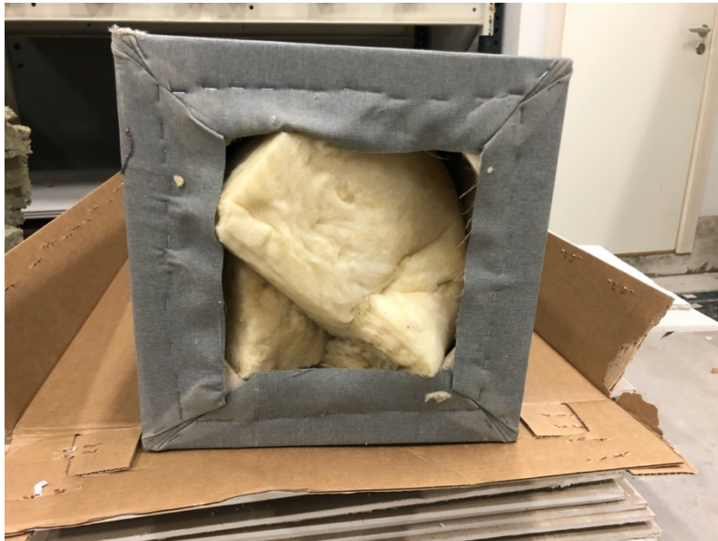
Figure 2: Inside space filled with mineral wool
