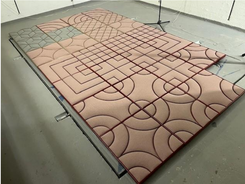
Figure 3. Mix of all available panels evaluated for sound absorption coefficient.
