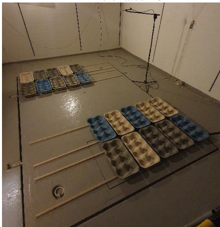
Figure A5:9: Eggbox measured as area, spaced apart.
