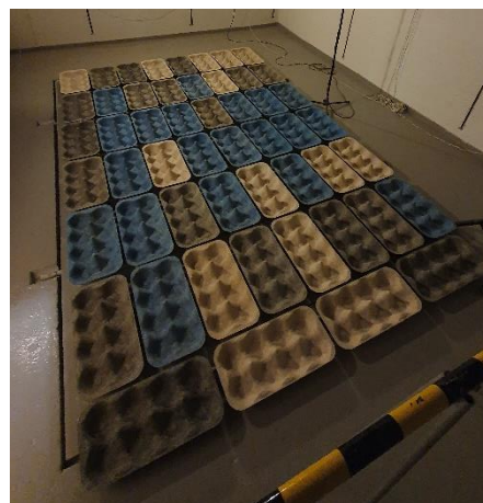
Figure A5:6: Eggbox spaced apart and elevated 20 mm.
